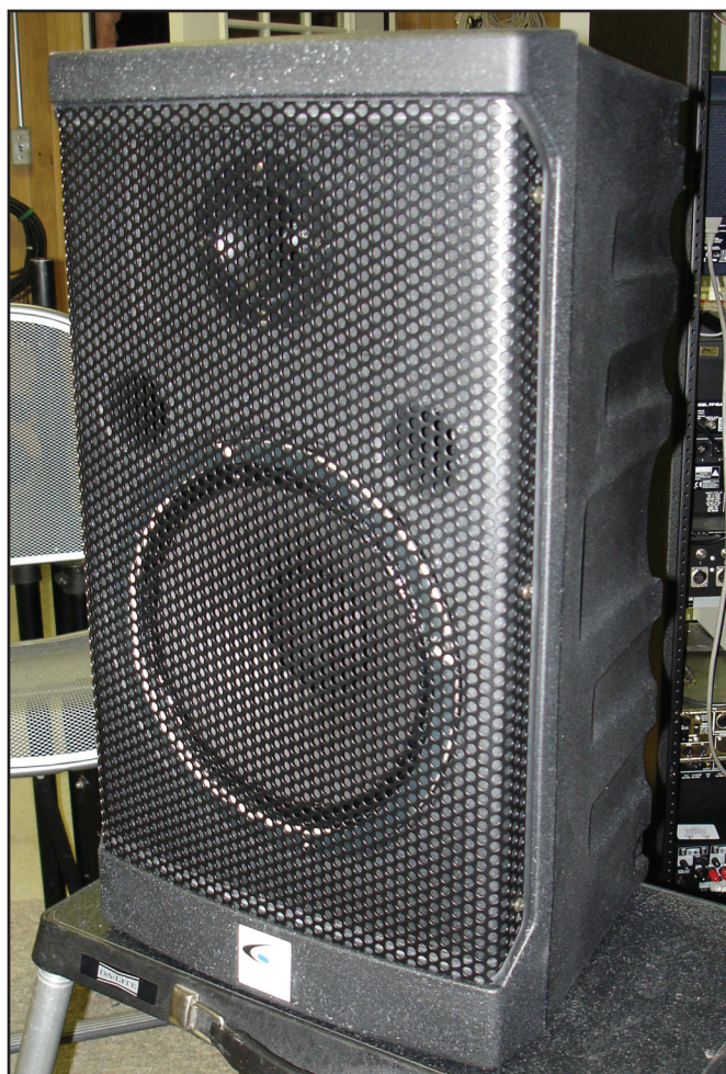
Figure 2 - The Lightspeed Delta X10 is a self-contained two-way powered loudspeaker. An internal battery provides ample time for a whole room survey. CD player (for stimulus) and wireless receiver are also available.
