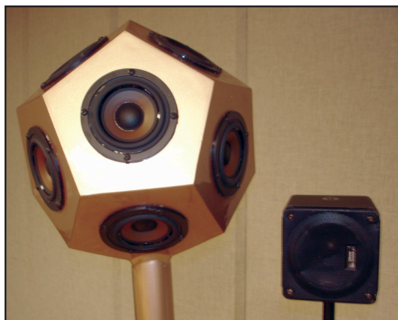
Figure 3 - An omni and talker loudspeaker can be used to assess the effects of different directivities on the IR. They connect to the external speaker jack on the X10, and the appropriate equalized sweep file is selected for playback.
