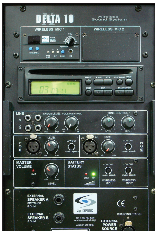
Figure 2 - The Lightspeed Delta X10 is a self-contained two-way powered loudspeaker. An internal battery provides ample time for a whole room survey. CD player (for stimulus) and wireless receiver are also available.
