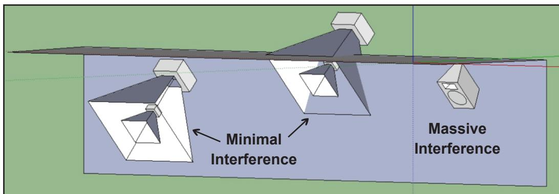
Figure 3 - Good physics and clever engineering can exploit the benefits of pattern control and boundary interaction avoid the destructive interference that plagues so many sound systems.
