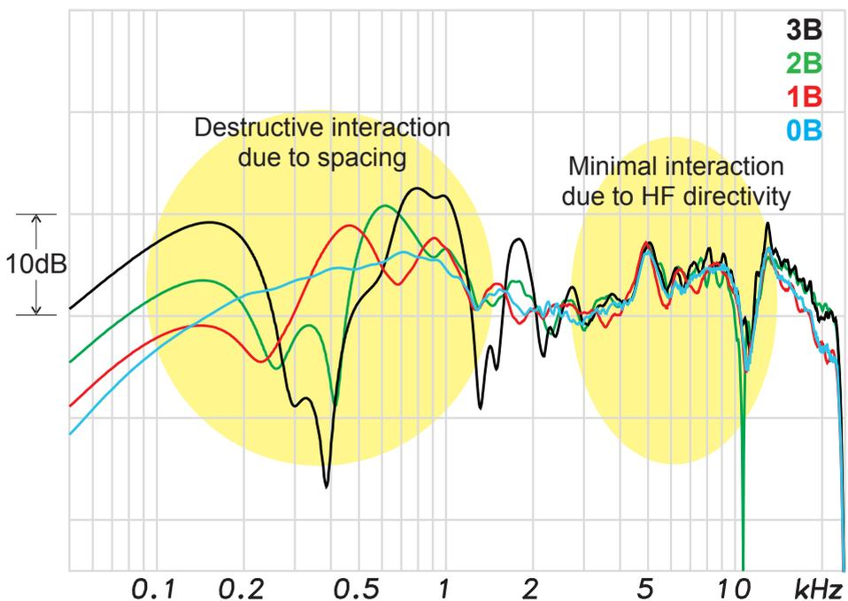
The device tested was a Bag End M-6 coaxial studio monitor - a bookshelf loudspeaker. Each measurement was made on the HF axis. The **1B** measurement was made with the loudspeaker's back against the floor. The **2B** and **3B** measurements were made with the loudspeaker at 45deg to the boundary, such as it might be mounted at the intersection of a wall and low ceiling.
