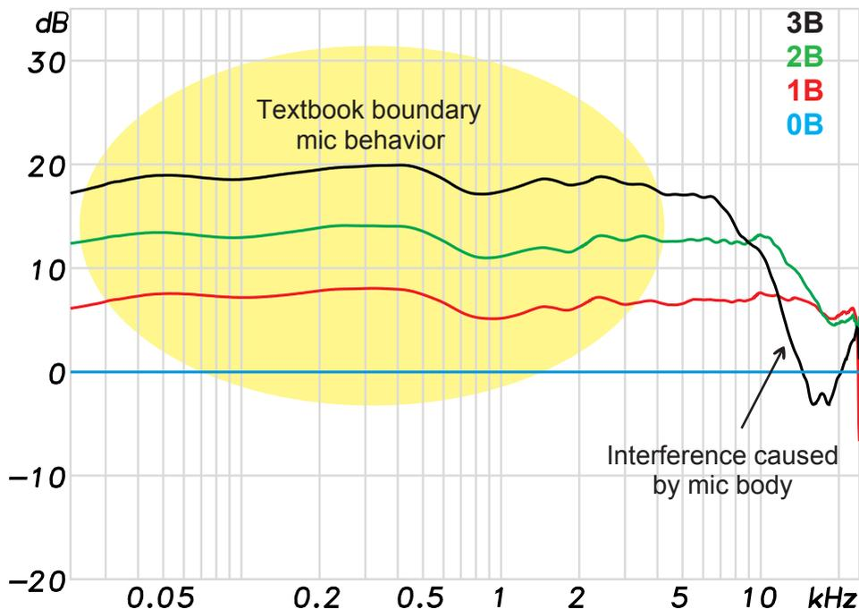
The device tested was a DPA 4007 microphone. A 6" coaxial loudspeaker was used as the sound source. The mic was placed on the HF axis and in the far-field for each measurement. The free-field measurement was used as a reference (0 dB line in the graph at left) and each subsequent measurement shows the *difference* caused by the boundary condition.
