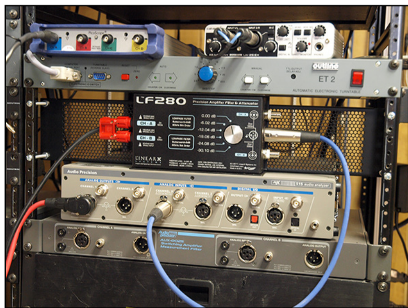
Figure 1 - The LF280 provides precise attenuation and low pass filtering.
